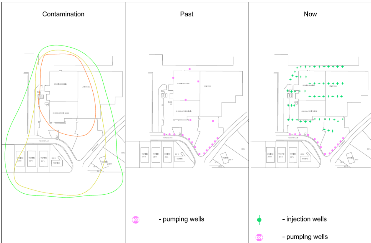
Figure 2 illustrates the extent of the contamination, along with the past and current remediation well systems in place. In the contamination illustration the green line represents the boundary of contamination with the lowest concentration at 10 microgram/liter (this is called the background value). The yellow line is 50 microgram/liter (this is called the soil remediation value) and the red line represents the highest concentration at 1000 microgram/liter.
