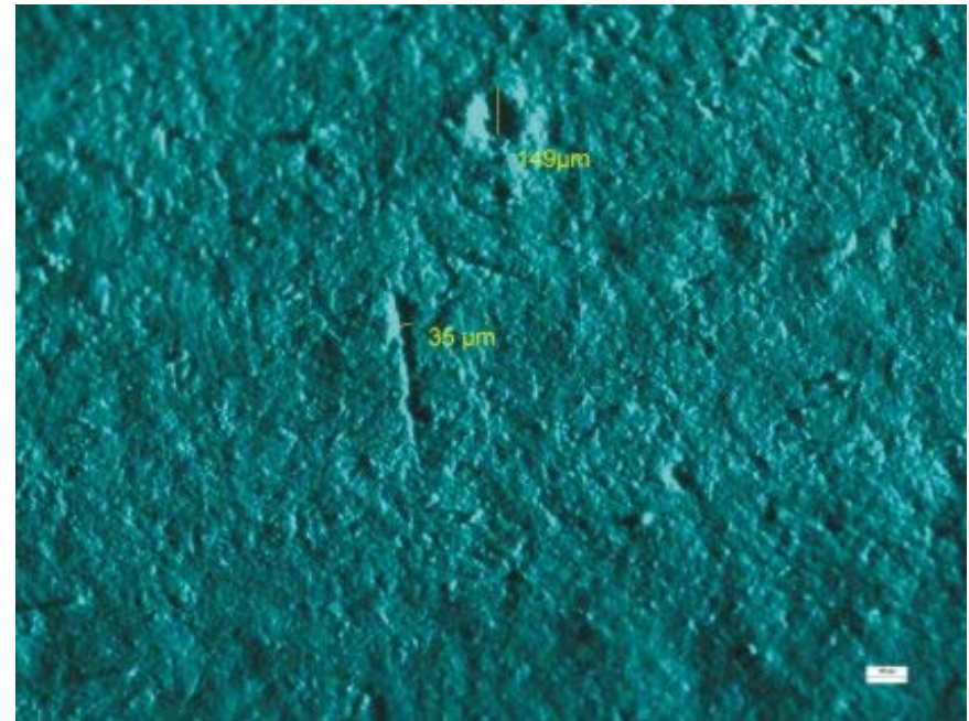
architectural coating after the process with two scratches
