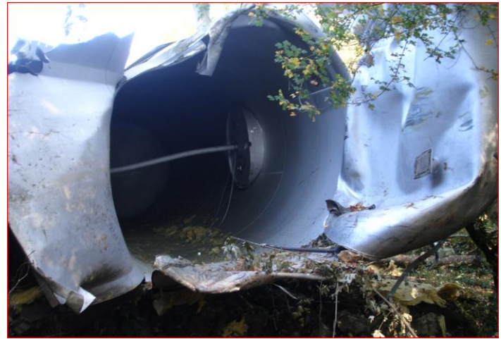
Empty RTC L4BH after high speed derailment
