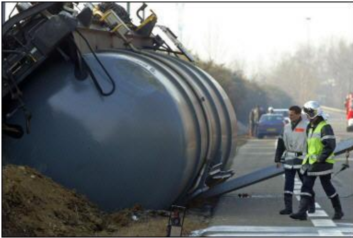
RTC falling down at low speed from shunting yard
