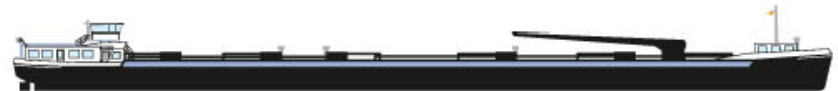
Large tank vessel Length 135 m - width 21.80 m - draught 4.40 m - cargo capacity 9,500 t
