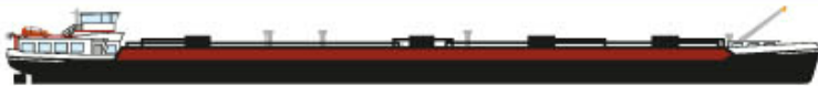
Standard tank vessel Length 110 m - width 11.40 m - draught 3.50 m - cargo capacity 3,000 t
