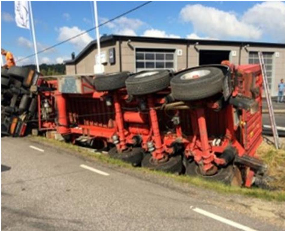
**Whilst exiting a parking zone of a cleaning station, the driver had to turn right onto the road. The turn was taken too sharply and the rear wheels passed onto the grass verge. The wheels slid and drove down the banking, leading to the tip and roll-over of the vehicle**
